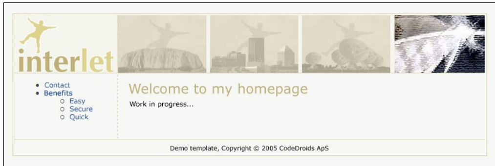
Illustration 26: OpenCms automatically constructs the navigation menu so the web user can navigate between the various pages on the site.
